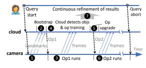
Figure 3: The workflow of a query's execution.
