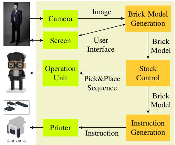
Fig. 2. The overview of system design: external input/output (left) and internal modules (right) including hardware (green blocks) and software (orange blocks).
