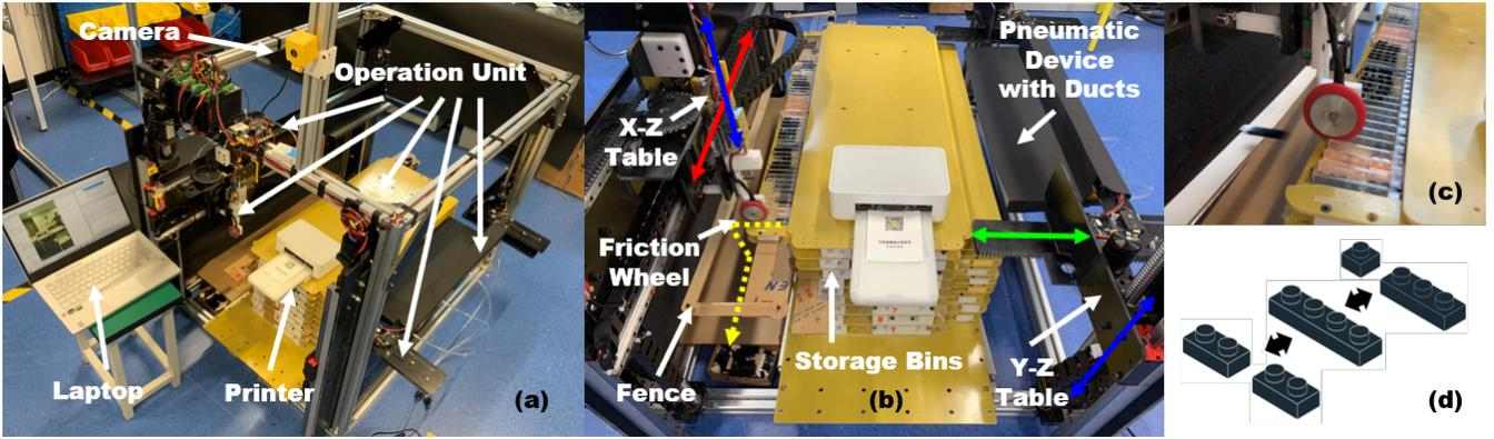
Fig. 3. Instances of hardware: (a) hardware system overview, (b) breakdowns inside the operation unit and a brick’s trajectory (yellow dashed) from the storage bin to the output box, (c), the instant of the friction wheel touching a black brick, and (d) alternative brick combinations for a  $1 \times 4$  plate.
