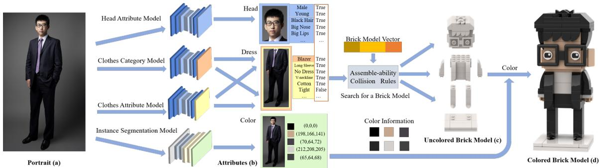
Fig. 4. Overview of our brick model generation pipeline. Given the input portrait (a), we use several deep neural networks to extract the attributes (b) to describe the human appearance shown in the image. Built on these attributes, we generate the corresponding uncolored brick model (c) by iteratively searching for brick component with the coordinate descent algorithm. Finally, we assign color to every brick to get the final brick model (d).
